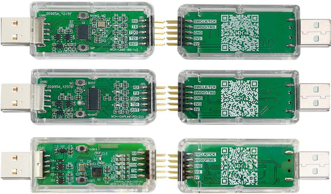
Figure 1 WCH-Link physical diagram
